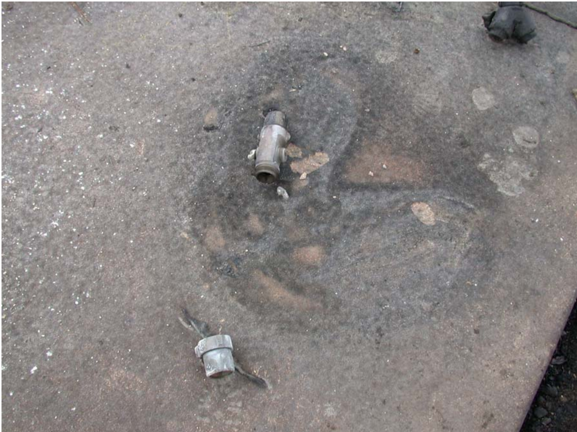
Burnt outline of first 100 feet hose pack dropped near the feet of Engineer Rucker on patio. In-line Tee visible in upper middle portion of photo.
