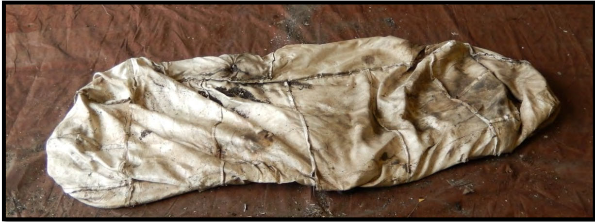
Figure 6. The burned remnants of a fire shelter that was recovered from the Yarnell Hill Fire deployment site shows signs of extremely high heat. The photo was taken during equipment inspection.
